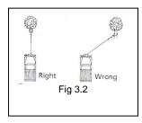
▲ CAUTION Do not winch from an acute angle as the wire rope will pile up on one side of the drum causing damage to wire rope and the winch. Fig 3.2
